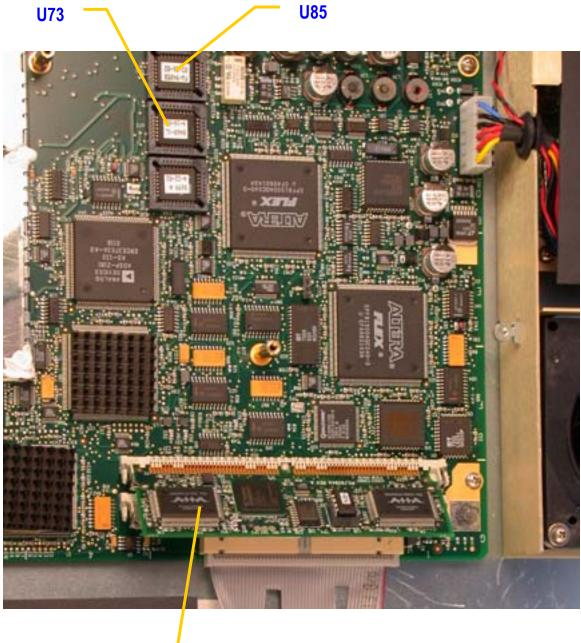
TURBO CODEC INSTALLED Figure 3
